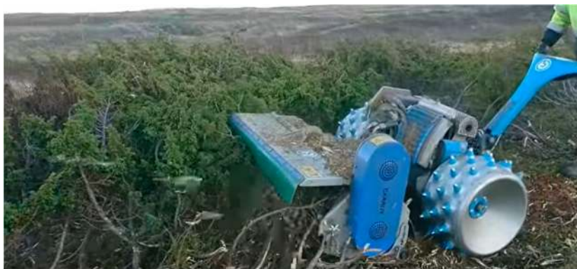
Figure 21. Mastication using a two-wheel tractor. Photo by Lauvrud Maskin. (Reproduced with permission).
