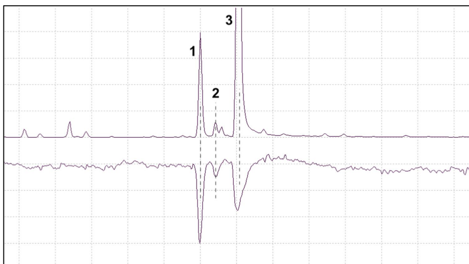
Fig. 6 GC-EAD analysis: the SPME sampling of a P. punctifrons male boring into the bark of a Norway spruce (TIC, upper trace) and the response from a P. poligraphus female antenna (lower trace). The antenna responded to (–)-(R)-terpinen-4-ol (1), α-terpineol (2) and (+)-(1R,2S)-grandisol (3)
