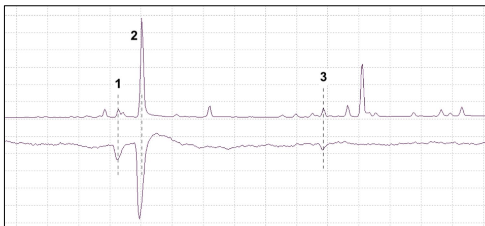
Fig. 3 GC-EAD analysis: the SPME sampling of a P. subopacus male boring into the bark of a Norway spruce (TIC, upper trace) and the response from a P. subopacus female antenna (lower trace). Antennal stimulants were grandisol (1), (Z)-DMCHE (2), and a host tree com-
