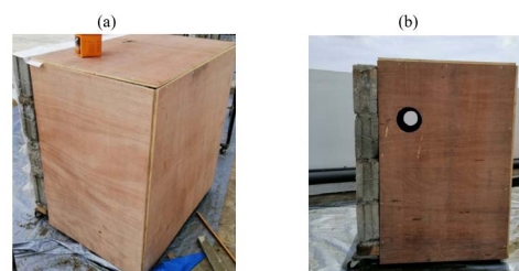
Fig 2. The exposed sides covered with plywood sheets: (a) after covering, (b) after cutting the openings.
