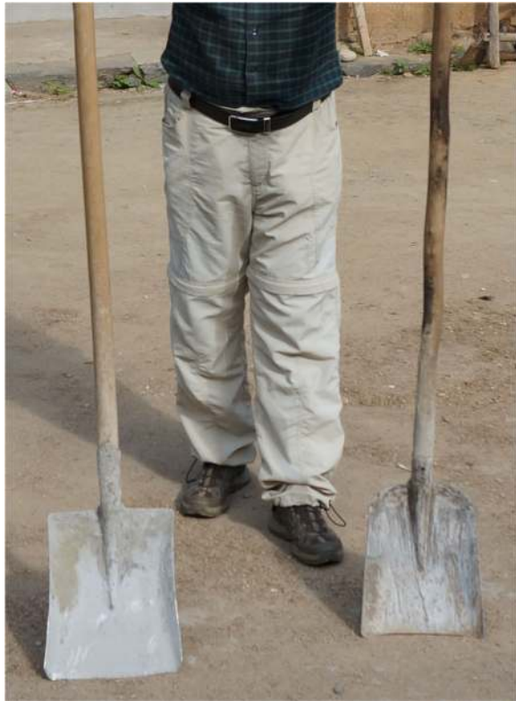
Fig. 4 Two spade handles – the one on the left made from Meliosma wood, the one on the right from C. kousa
