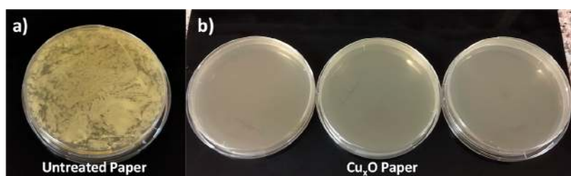
Figure 4. Antifungal activity of \text{Cu}_x\text{O} paper. (a) Proliferation of C. albicans on the untreated paper surface. (b) Agar plate photos showing \text{Cu}_x\text{O} paper killing all C. albicans ( n = 3 ).
