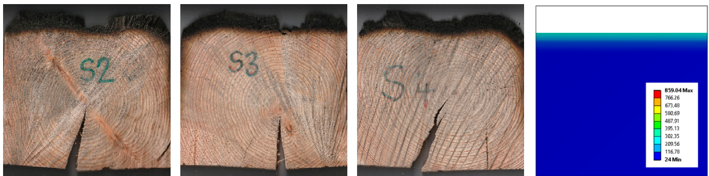
Figure 8. Cross section of samples: comparison of results from medium scale fire tests and simulation.
