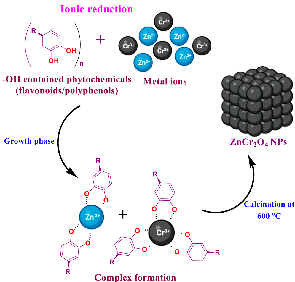
FIGURE 7 A potential mechanistic approach for the environmentally benign generation of ZnCr 2 O 4 NPs.
