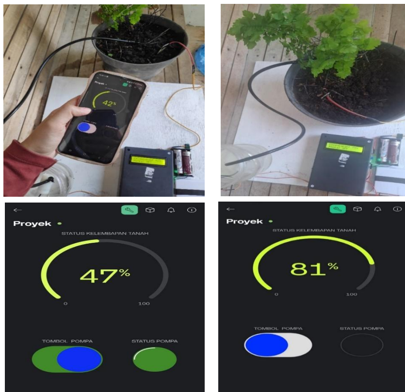
Figure 5. Testing of Soil Moisture and Blynk Sensors on Maidenhair Ferns
