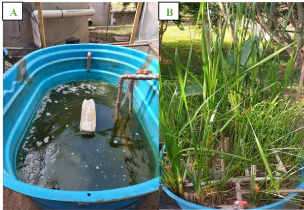
Figure 2. Upper view of the Integrated Treatment System. A) Microalgae Unit B) Constructed Wetland.
