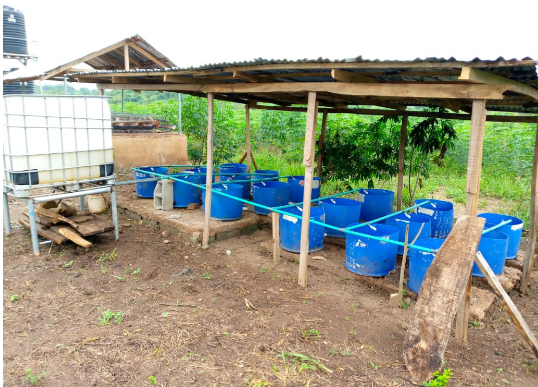
Figure 2. Setup of vertical subsurface constructed wetlands used to treat wastewater under the conditions of seasonal variation, treatment type, and retention time.
