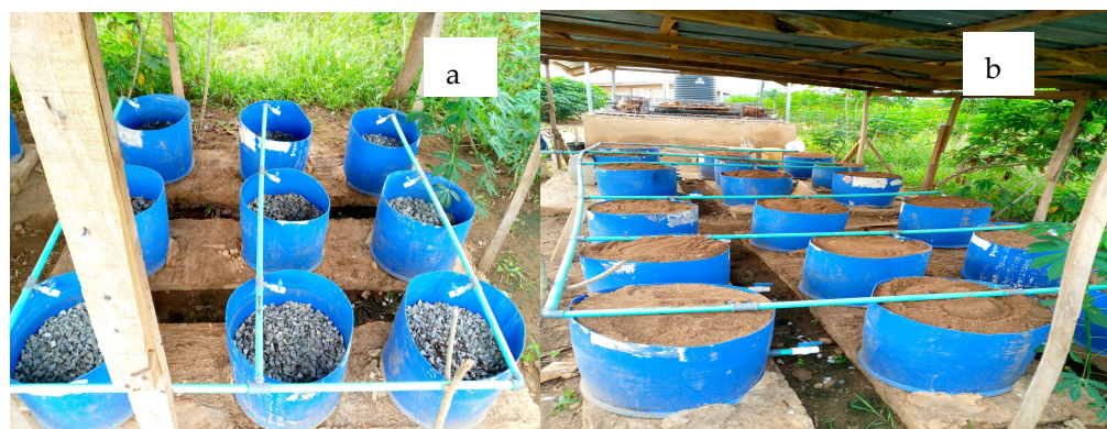
Figure 1. Vertical subsurface wetland filled with coarse gravel (a) and coarse gravel + sand (b).
