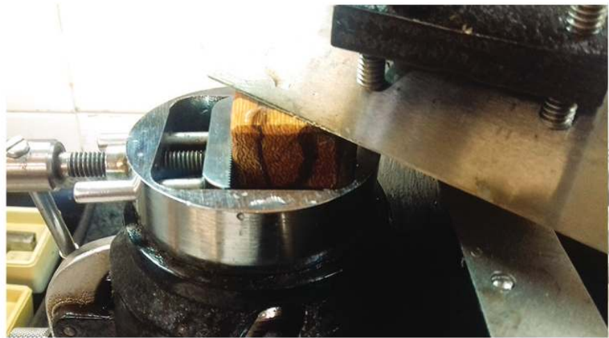
Figure 12. Flattening of the surfaces of the Angelim Rajado sample in the slide microtome.
