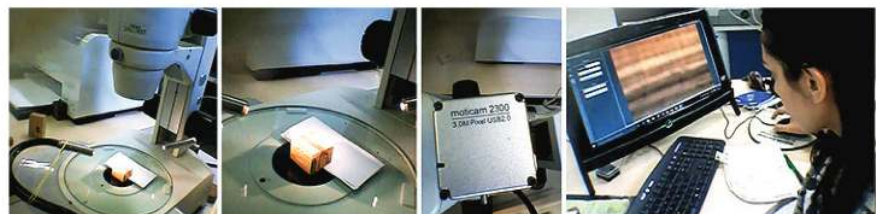
Figure 13. Capture of digital images of the macrographic anatomical elements of Angelim Rajado wood.
