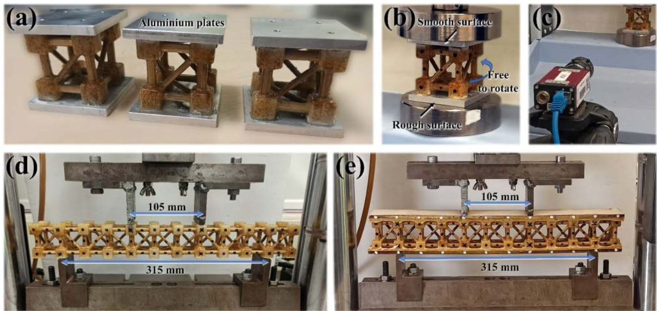
Fig. 12 Insights on the mechanical characterisation of the trussed structures: a metastructure trussed cells attached to aluminium plates, b compression test of the trussed cell, c video gauge, d four-point bending of the trussed beam, and e four-point bending of the sandwich beam
