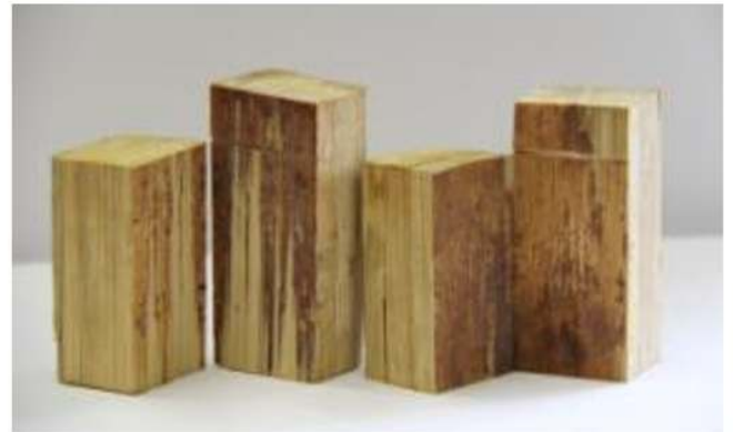
(b) Shear parallel to glue surface of GLB.
