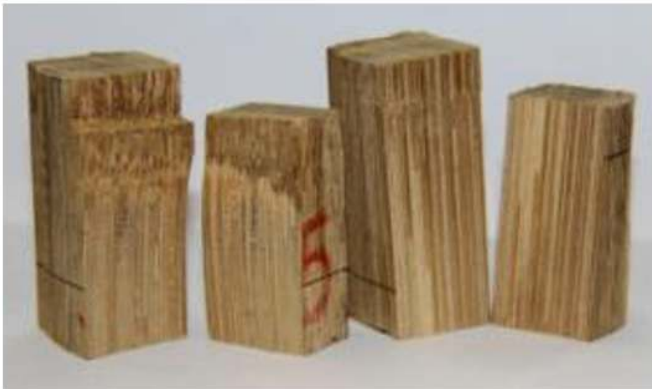
(a) Shear parallel to grain of bamboo.
