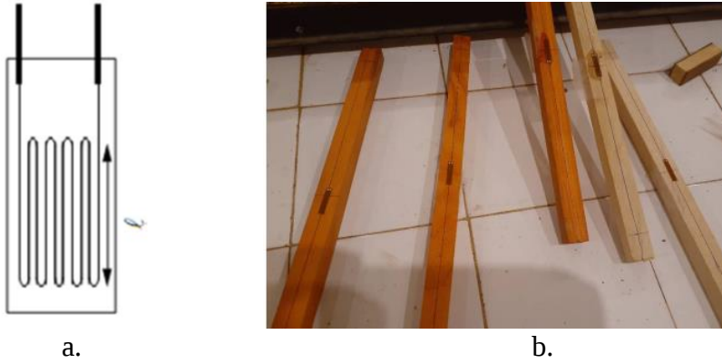
Figure 6. a. Strain gauge; b. Samples carrying two gauges.
