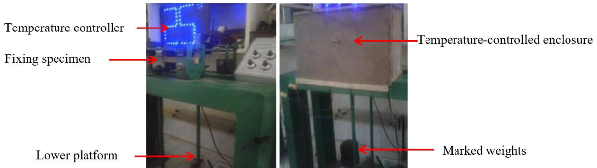
Figure 7. Experimental protocol for determining Young's modulus as a function of temperature (Foadieng et al. 2021).
