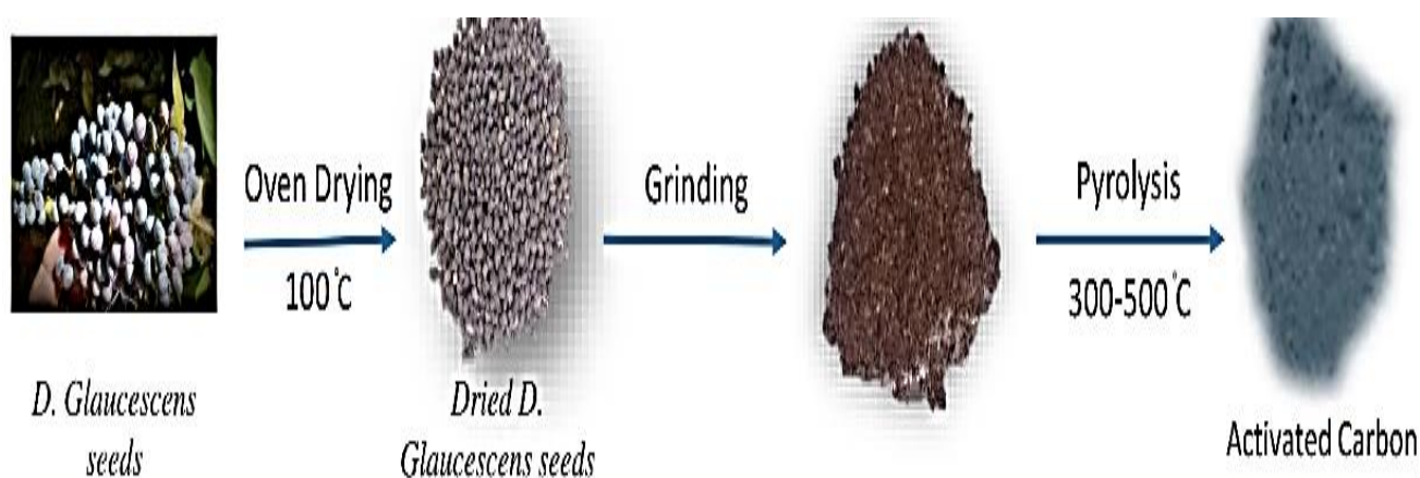
Figure 2. Schematic diagram for DGAC preparation
