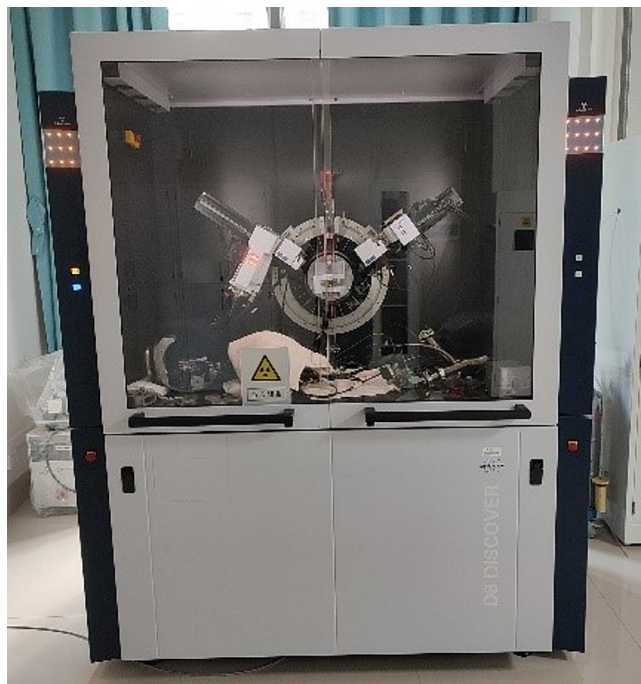
Figure 3. Bruker XRD Goniometer (D8 DISCOVER).
