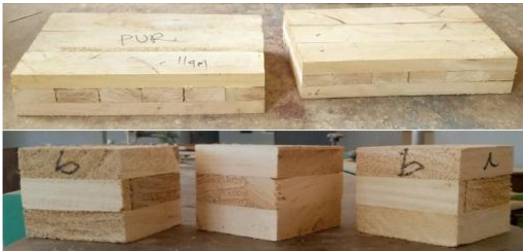
Figure 5: The 3-layer CLT panels and the extracted specimens
