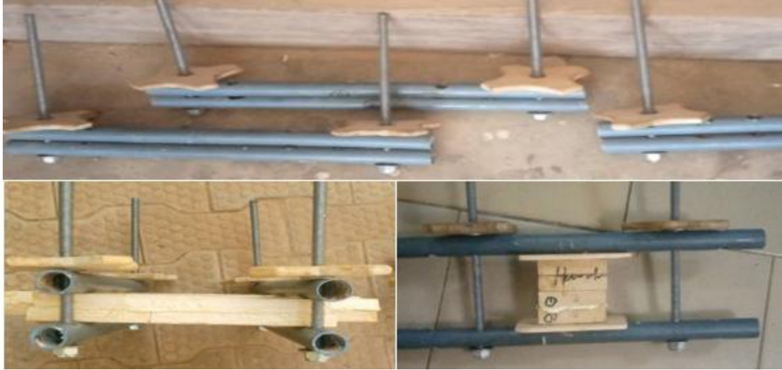
Figure 2: Improvised clamping device for pressure application (Yau et al., 2024d)
