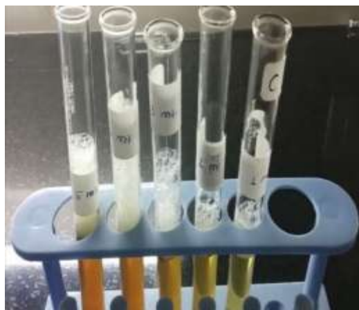
Figure 4: Foam Persistence Test
