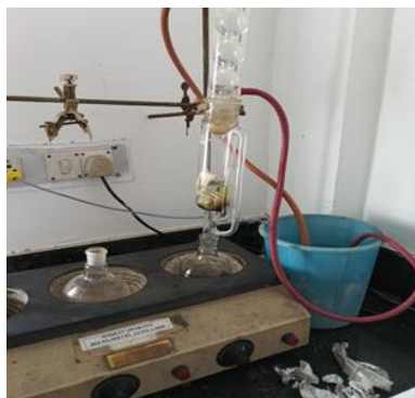
Fig 3. Soxhlet Extraction of Parsley Plant
