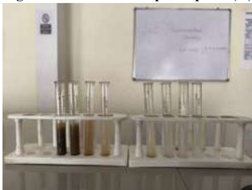
Fig. No. 13- Serial dilution of soil sample
