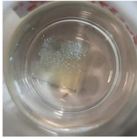
Fig. 4: Picture of the IAGl triple layer after 4 days of submersion in PBS at 37 °C. Clear signs of degradation can be seen, as several flakes have been removed from the glass surface and have dispersed in the solution.
