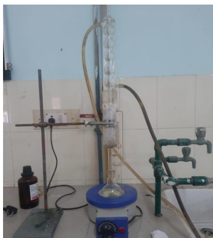
Fig 1. Grape Seed Extraction by Soxhlet Apparatus
