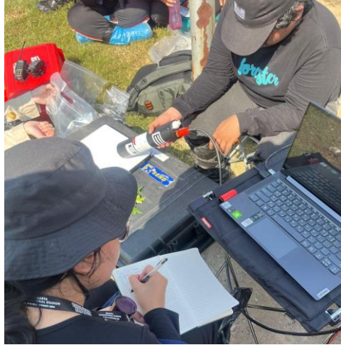
Figure 3. Collection of spectral reflectance data of mangrove leaves in the Mundupesisir area, Cirebon.
