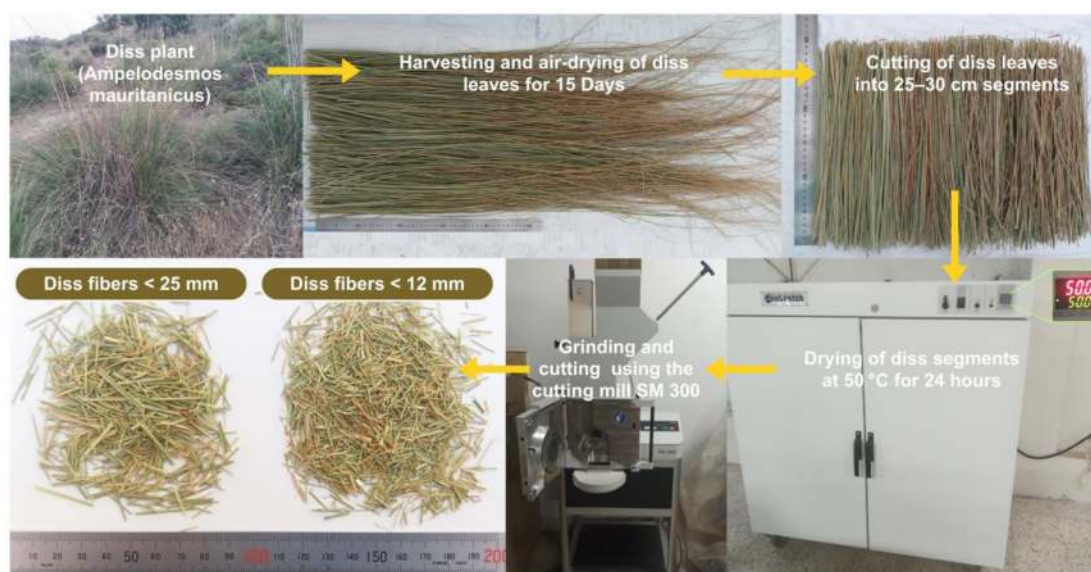
Fig. 1. Preparation steps of diss Fibers.
