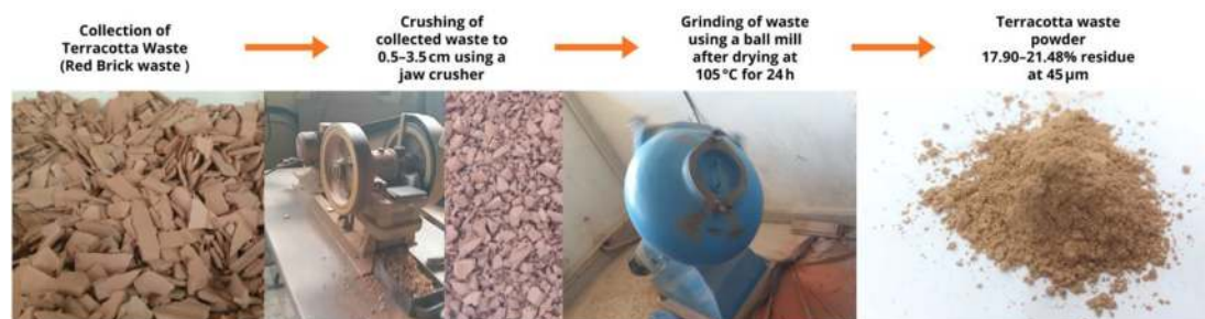
Fig. 5. Preparation process of terracotta waste powder (TWP).
