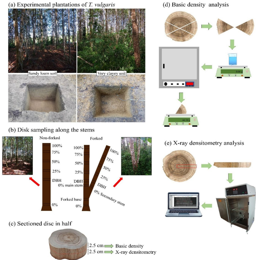
Fig. 2 Experimental plantations of T. vulgaris evaluated on soils with sandy loam texture and very clayey texture (a), disk sampling along the stem of non-forked and forked trees (b), disks split in half generating duplicates with \approx 2.5 cm thickness (c), basic density analysis (d), and X-ray densitometry analysis (e)
