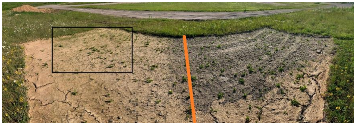
Fig. 6 - Panoramic view of 15 x 7 ft study area with orange line dividing sludge test side using 100% sludge with embedded seed (left) and Celumulch test side (right) using 100% Celumulch and embedded seed after 12 days. Both sides contained grass growth composed of 40% Creeping Red Fescue ( Festuca rubra ), 30% Perennial Ryegrass ( Lolium perenne ), and 30% Kentucky Bluegrass ( Poa pratensis ).
