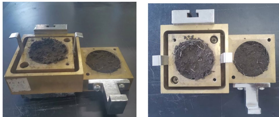
Fig. 7. Shear failure of specimen.
