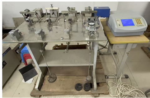
(a) STSJ-5A intelligent electric four-unit direct shear apparatus
