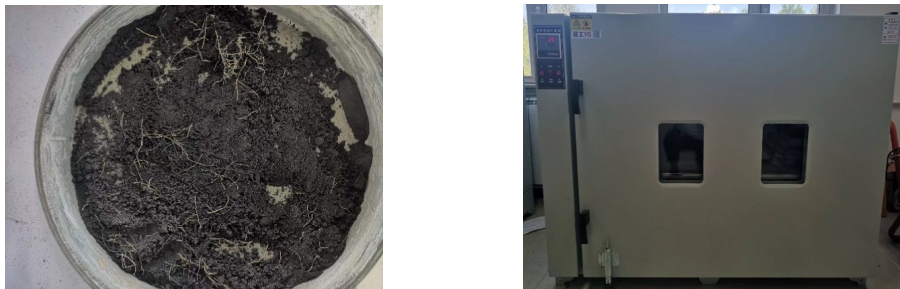
(a) Remodelled root-soil composite (b) XMA-2000 electric blast drying oven
