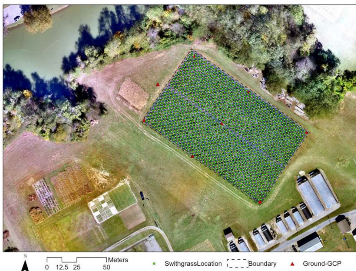
Figure 6. Field map of the switchgrass locations and ground control points (GCP). The color map is the composite of the R, G, and B bands collected with the Zenmuse camera. A total of eight control points (including one ground station), as shown in red triangles, were surveyed in the field. The Global Positioning System (GPS) antenna was manufactured by CHC Navigation (Shanghai Huace Navigation Technology Ltd., Shanghai, China). It is a static GPS, post-processing used Online Positioning User Service (OPUS) to resolve the high-accuracy positioning. The eight control points were collected in the field from 5 to 30 September 2019. The field ground- and UAV-based data for the four sustainability traits were collected at several time points (Table 4). Data collection for chlorophyll was at one time-point (mid-season), for rust disease at one time-point (mid-season), and for nitrogen and lignin at two time-points (mid-season and end of the season).
