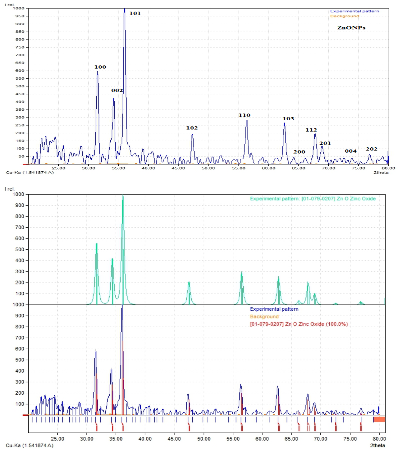
Fig. 5. XRD pattern of green synthesized Zinc oxide nanoparticles.
