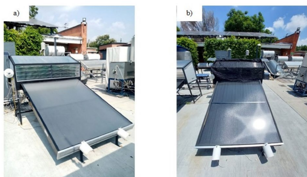
Fig. 1 Mixed-type solar dryer used in the drying process of avocado leaves a) without mesh shade and b) with mesh shade
