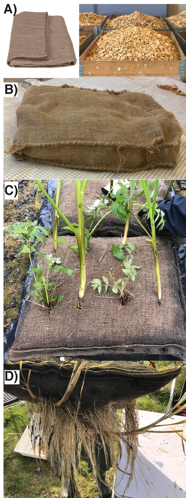
Fig. 1. Construction and pictures of a woodchips-based floating bed (WFB), A) jute sheet and freshly cut birch woodchips, B) sack made of woodchips and jute sheet, C) Glyceria maxima and Filipendula ulmaria planted on a WFB, D) plant root growth below a WFB at the end of the experiment.
