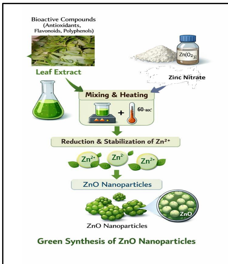
Figure 1. Procedure for the synthesis of ZnO nanoparticles
