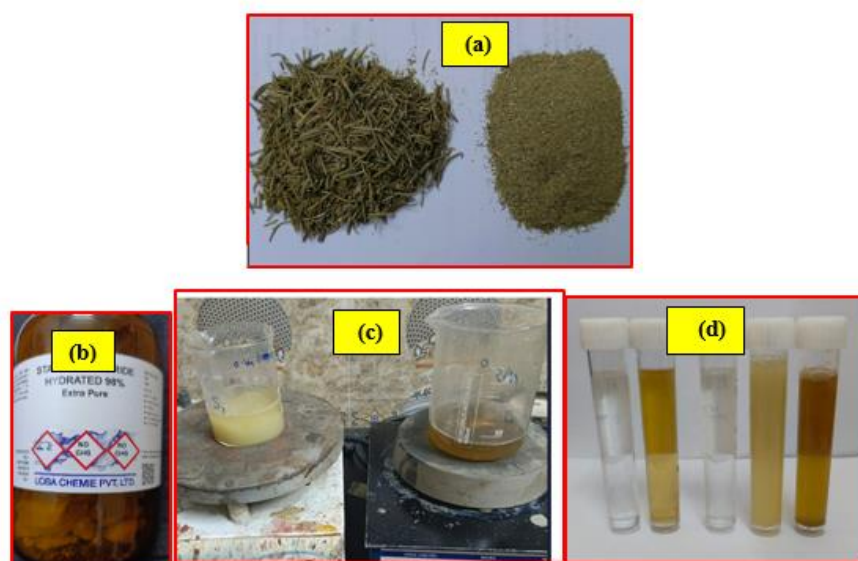
Fig.1. preparation of SnO 2 by green synthesis method at different concentration: (a) The Salvia rosmarinus (b) SnCl 4 • 5H 2 O (c)SnO 2 at 0.1M and 0.2M during work under 80C. (d) from left: distill water , Salvia rosmarinus extract , SnCl 4 • 5H 2 O solution ,SnO 2 colloidal at 0.1 and 0.2M respectively.
