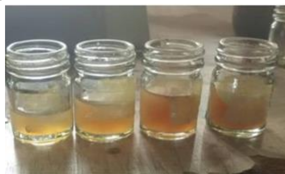
Figure 1: Visual indicator of the reduction process confirms the formation of AgNPs (left to right).
