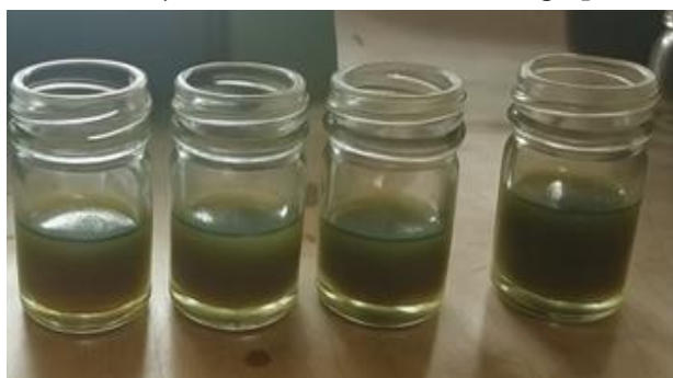
Figure 1: Visual indicator of the reduction process confirms the formation of AgNPs (left to right).
