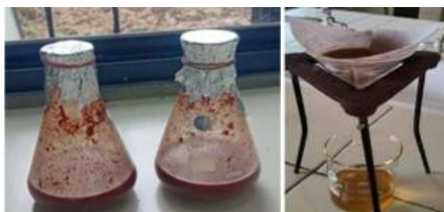
Figure 1: Extraction of Arjuna Bark and Reetha fruit by maceration method
