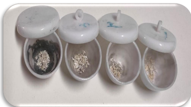
Figure 3: The samples, after ashing, were carefully removed from the crucibles and weighed.
