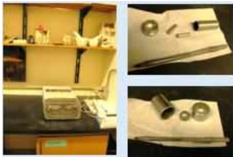
Retsch mill grinder and stainless steel grinding vessels
