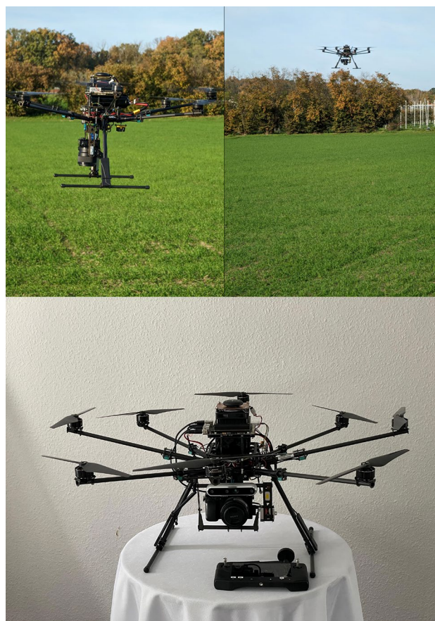
Fig. 1 The OktopusXL flying platform utilized for data acquisition in this study. It features eight propellers and employs the Pixhawk autopilot hardware. The octocopter is equipped with an HD video transmission and control system, enabling it to stream control, video, and drone telemetry data via a 2.4 GHz connection to a remote control unit
