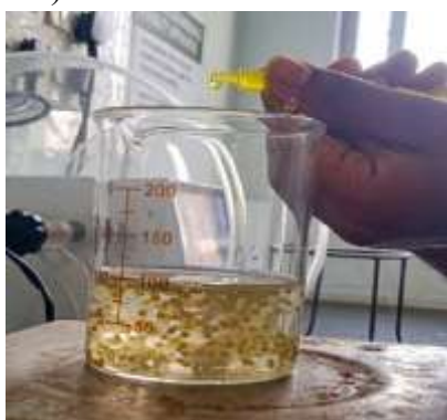
Fig.7: microbeads loaded with Syzygium cumini (Jamun) leaf extract
