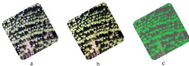
FIGURE 5. Image enhancement and classification: (a) the orthophoto image of the sample plot generated by oblique photogrammetry, (b) an enhanced view of the image, (c) the result of tree crown and ground classification (green is the tree crown, translucent gray is the ground background).
