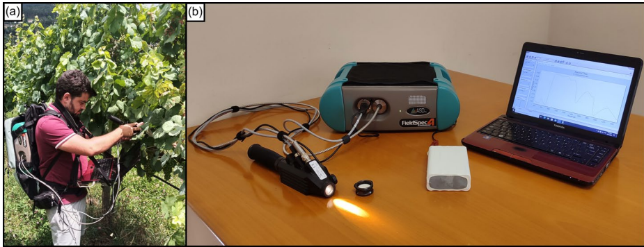
Fig. 2 Field spectral data acquisition performed directly on grapevine leaves (a) and spectroradiometer setup (b)
