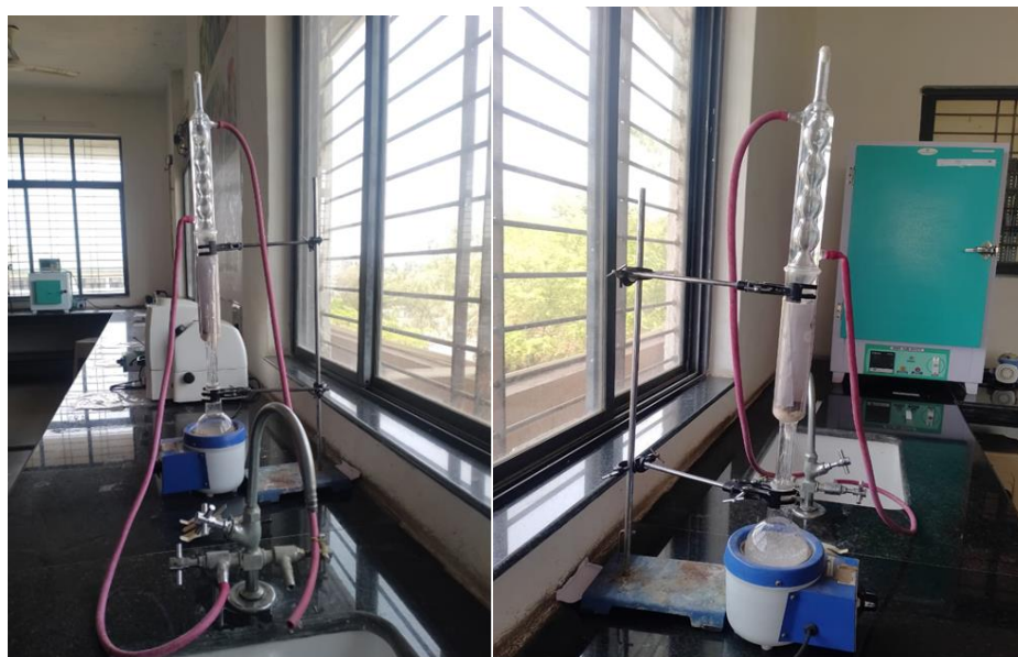
Fig. No. 4: Soxhlet Extraction.
