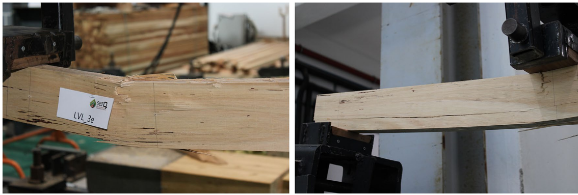
Fig. 3 Failure modes observed from edgewise bending tests on LVL specimens: compression folds at the upper side combined with failure by tension (left); shear combined with tension failure (right)
