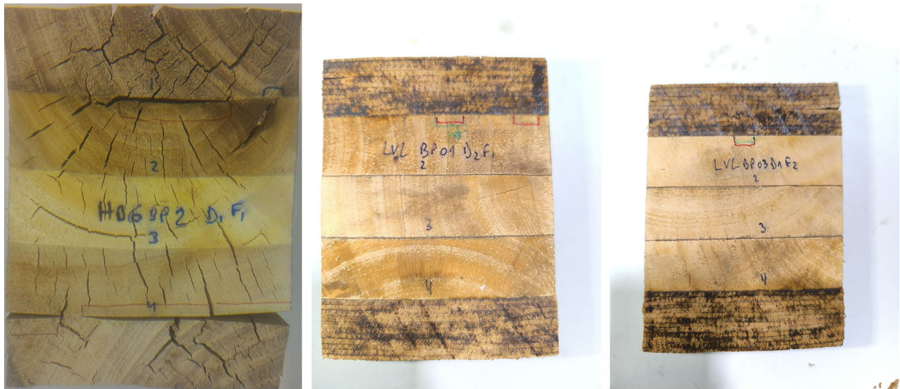
Fig. 15 Specimens after delamination test: left—HBGBP (Martins et al. 2020); centre and right—HLVL-BP
