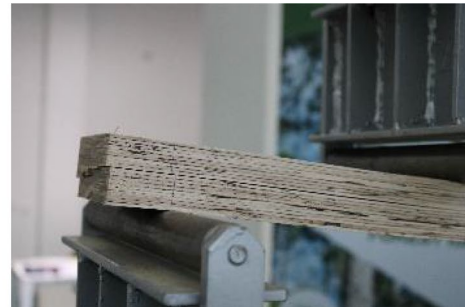
Fig. 4 Load vs deflection curves from flatwise bending tests (left) and shear failure mode observed (right)
