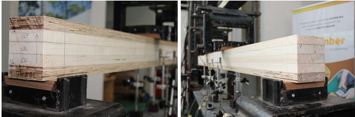
Fig. 8 Lay-up of HLVL-BP (left) and HLVL-4BP (right)
