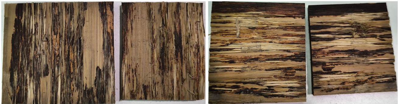
Fig. 6 LVL bonding quality: wood fibre failure above 70%
