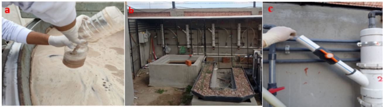
Fig. 1 a Arma factory for industrial oily wastewater. b Effluent wastewater from the UASB unit. c The modified UASB reactor: inoculating the immobilized Phragmites australis biochar with Streptomyces hydrogenans
