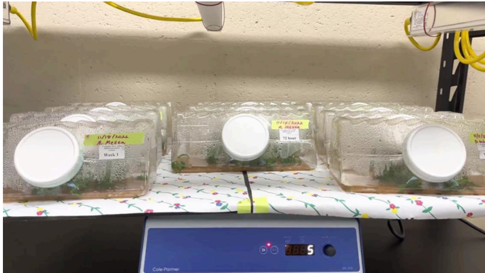
Figure 8. Southern Sun BioSystems vessels on rocking platform with an articulated shelf (5rpm) exposed to 20 \mu\text{mol/s/m}^2 , 16h/day at 24^\circ\text{C} .
