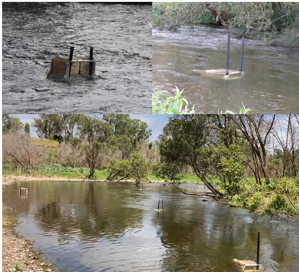
Fig. 2. Propagule dispersal nets deployed at different depths and flow velocities across the river channel.
