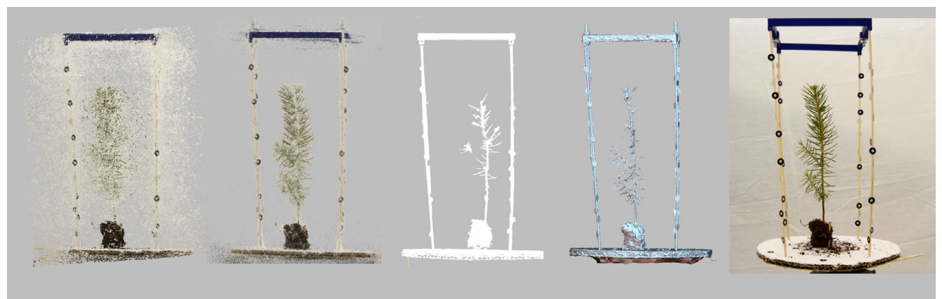
FIGURE 6 | Generated point clouds. Comparison of the resulting dense point cloud from different photogrammetry software and 3D scanning. From left to right: Agisoft, Meshroom, RealityCapture, Shining 3D and the original seedling.
