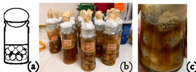
Figure 2. Reactor prototype of 250 ml. (a) schematic picture, (b) photo of the systems, (c) details of biofilm.
