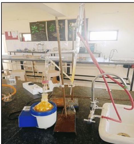
Figure 4 Clavenger assembly for extraction
