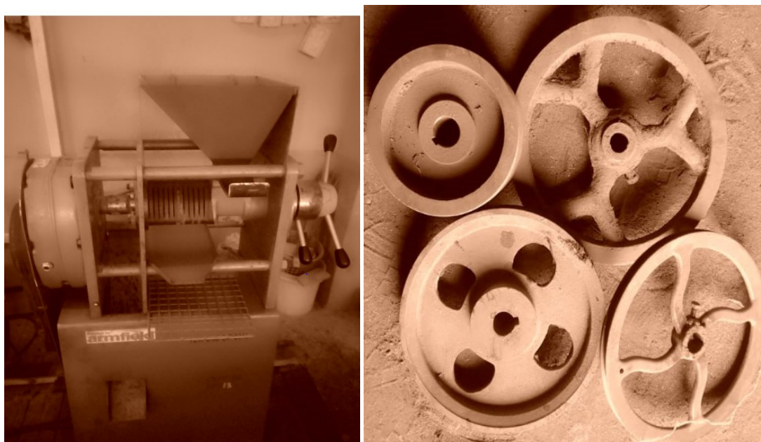
Plate 1: Armfield-FT28 screw press (Savoire et al., 2012). Plate 2: Photograph of the four pulleys used to vary the main shaft speed
